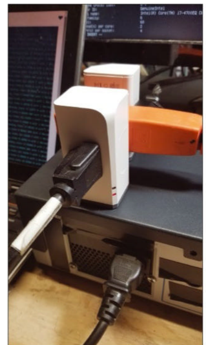
Figure 2: Bare metal Kubernetes host powered by Sonoff switch with power readings scraped into Prometheus.
