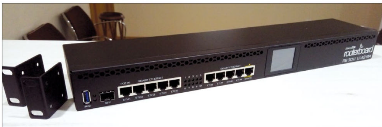
Figure 1: MikroTik equips their low-end SOHO routers with the same firmware they use for their more powerful products. Pictured is a RouterBOARD RB3011UiAS-RM intended for a network rack – clearly not a router designed for home users.
