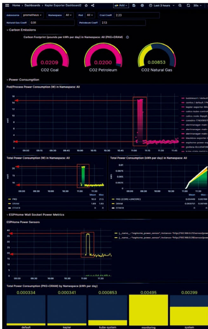
Figure 8: Kepler's Grafana dashboard shows that Kepler has detected the power increase caused by the test bubblesort workload on the Haswell node.
